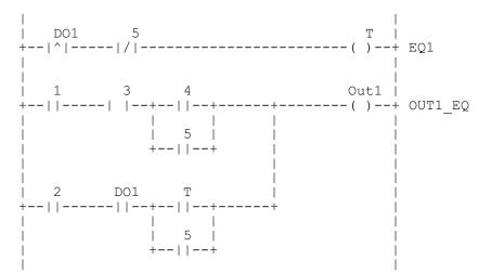
First, instantiate two DI blocks and a DO block. Set the DO channel to 9. Set the Auto DI channel to 2 and the Contactor DI channel to 5. Use appropriate configuration for the other data in the blocks, such as Tag.
